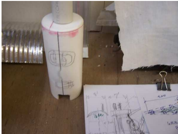
Boiler roughed out for rivet overlays.
