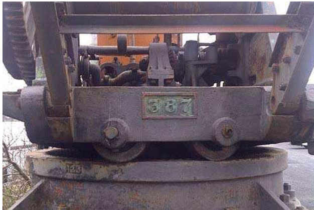
Trunnions and bearing ring detail.
